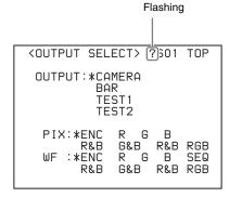
2 Turn the CONTROL knob to change the displayed page to the desired page, then press the CONTROL knob.
